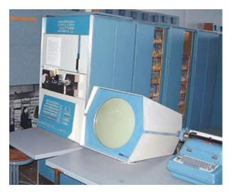
Fig. 1. The console of PDP-1 computer. See the large CRT display and an IBM Selectric typewriter for interactive use of the computer. [Courtesy: Image reproduced with permission from http://edthelen. org/comp-hist/vs-decpdp-1.jpg]
